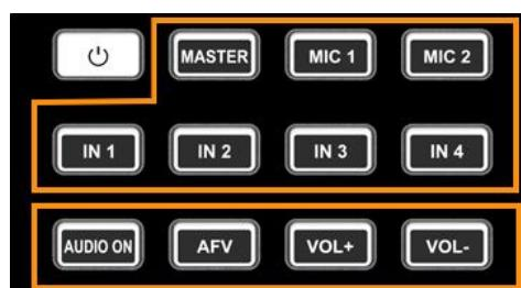
Part A is for selecting one audio to be configured, including Master, MIC 1, MIC 2, IN 1, IN 2, IN 3 and IN 4.
