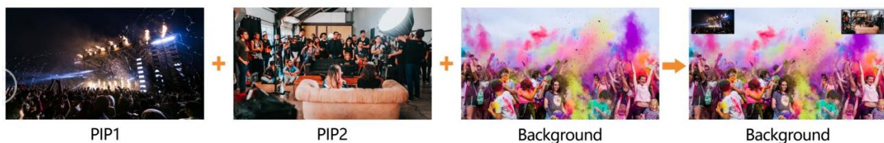
The video switcher supports two groups PIP or one POP. When press PIP1 or PIP2 button, there will be a small image display on the top left corner of PVW window. Press the Menu knob and choose the PIP setting interface, user can set parameters including position, size, border etc. PIP1 supports 0°, 90° and 270° rotation.
