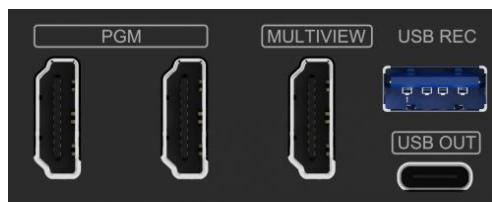
SHARK S4 has 3 HDMI output and 1 USB output. The three HDMI outputs are default as 1 Multiview out and 2 PGM out . All outputs also can be defined as an AUX OUT from IN1, IN2, IN3, IN4, PVW, PGM, Clean PGM, Color Bar and Multiview out.
