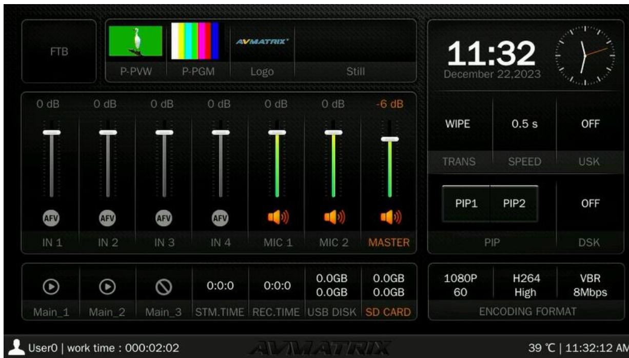
The information of user name, working time, CPU working temperature, system time keeps displaying in the bottom of the Status/Menu page.
