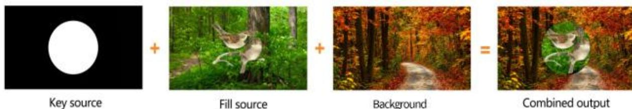
Luma key provides a way to composite a Text clip over a background clip based on the luminance levels in the video. Turn on the Luma Key, a color from the key source will be removed, revealing another background image behind it.
