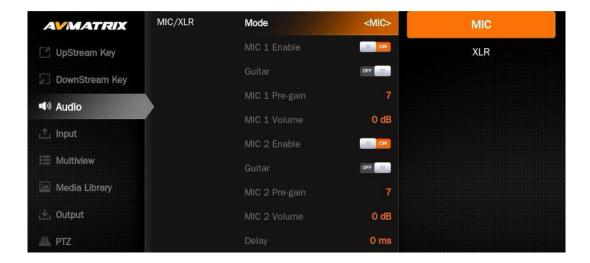
The S8X mixing function only supports mixing two channels. If there is an HDMI signal with 7.1 channels and you need to output 7.1 channels, you can select the surround sound pass-through function of the input. The HDMI output of PGM will include the last 6 channels of the input source and the first two channels of the mix.
