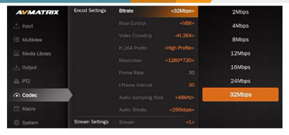
The encoding frame rate automatically follows the HDMI out frame rate and can be selected in the output format settings.
