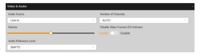
**Audio Source:** Select either HDMI embedded audio or analog audio input. HDMI embedded audio is used by default.
