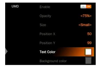
The UMD content for each HDMI input can be set from the on-screen menu. The user can use a virtual keyboard and rotary button to rename the UMD content for each window. The UMD content can be up to 10 characters long. Below image as an example, rename the IN1 to CAM1.
