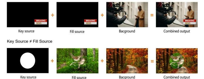
Switching a video with background to PVW window, and turn on the Luma Key. Press the menu knob to enter the setting interface. Under Luma Key sub-menu, user can assign the fill and key source from various options including Black/ Color Bar/ Color1/ Color 2/ IN1/ IN2/ IN3/ IN4/ Image (import from USB disk). Configure and adjust the Key parameters including Clip/Gain/mask to achieve
